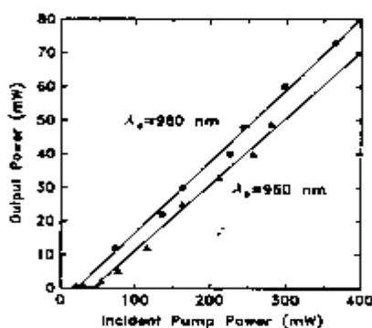
Fig. 3. Output power from the  $\text{Er}^{3+}:\text{Yb}^{3+}$ :phosphate glass laser pumped by a  $\text{Ti}:\text{Al}_2\text{O}_3$  laser as a function of the input power incident upon the rear face of the laser disk for a pump-light wavelength  $\lambda_p$  of 980 and 960 nm.
