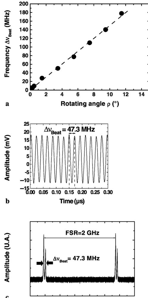
FIGURE 2 Characterization of laser in dual frequency regime: (a) evolution of beating frequency  $\Delta\nu_{\text{Beat}}$  versus the rotating angle of the second quarter-wave plate  $\varrho$ ; (b) temporal signal; (c) optical spectrum
