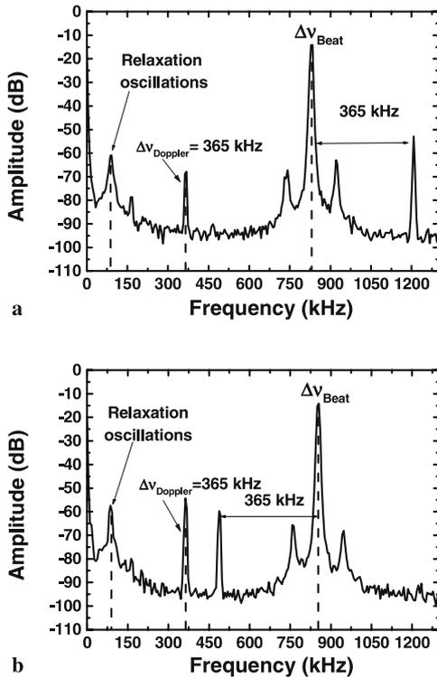
**FIGURE 3** Radio-frequency spectra of the detected signal in heterodyne detection with a simple linear polarizer (set-up (a) of Fig. 1): (a) disc turning clockwise; (b) disc turning anticlockwise
