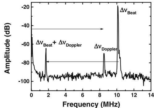
FIGURE 5 Radio-frequency spectrum with a Faraday rotator and a large beating note between the two modes to show the extension of the velocity range measurement
