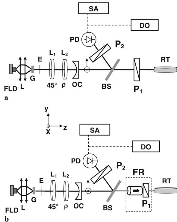
**FIGURE 1** Experimental set-up: DO, digital oscilloscope; SA, rf spectrum analyser; FLD, fiber laser diode; G, Yb:Er glass; E, etalon; OC, output coupler; L, lens;  $L_1$ ,  $L_2$ , quarter-wave plates ( $\lambda/4$ ); BS, beam splitter; PD, InGaAs photodiode; FR, Faraday rotator; RT, rotating target
