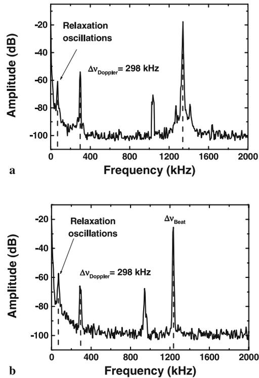
FIGURE 4 Comparison between the rf spectra of the detected signal without Faraday rotator (a) and with Faraday rotator (b)
