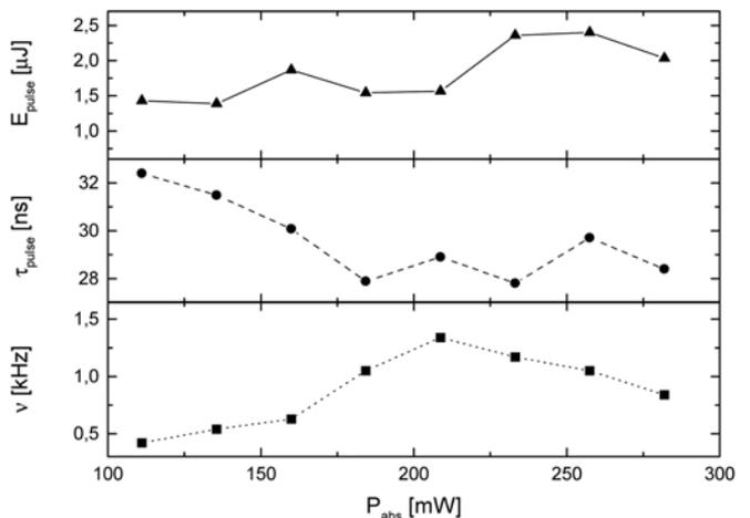
**Fig. 2.** Pulse energy, pulse width and repetition rate for phosphate glass with 300- $\mu\text{m}$ -thick absorber
