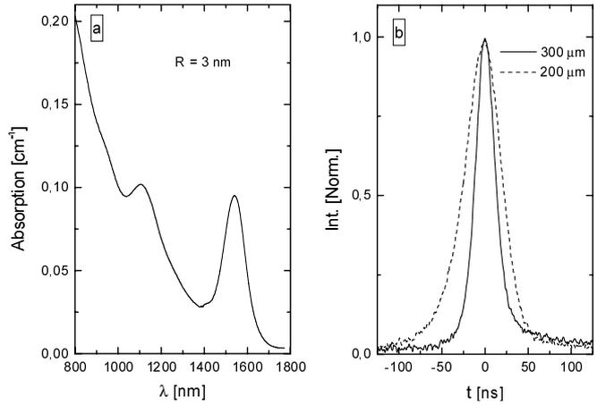
**Fig. 1.** a Absorption of PbS doped glass. b Pulse duration for different absorber thickness
