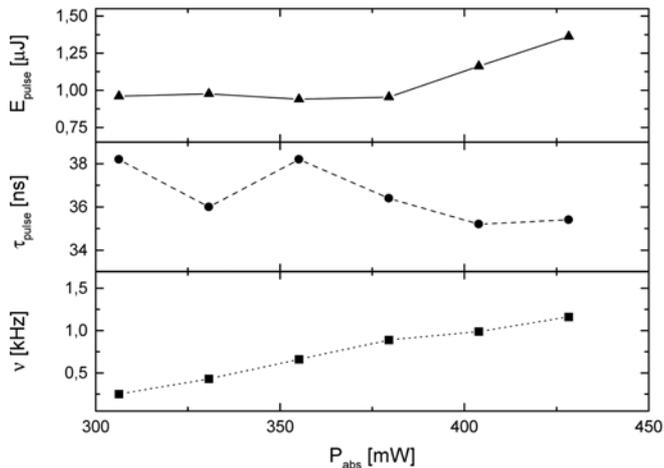
Fig. 3. Pulse energy, pulse width and repetition rate for fluoride phosphate glass with 300- $\mu\text{m}$ -thick absorber
