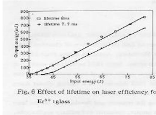
Fig. 6 Effect of lifetime on laser efficiency for  $\text{Er}^{3+}$  glass
