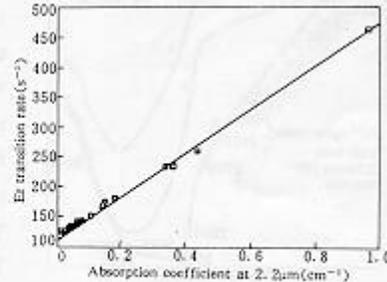
Fig. 5  $\text{Er}^{3+}$  transition rate as a function of absorption coefficient at 2.2 μm
