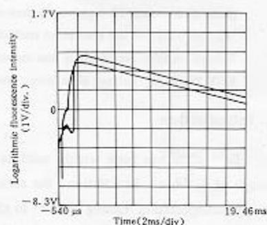
time, from these different excitation sources are shown in Fig. 2. The same slope was observed for the upper trace excited by the free running laser as the lower trace by Q-switched laser.
