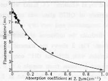
Fig. 4 Relationship between fluorescence lifetime and absorption coefficient at 2.2 μm
