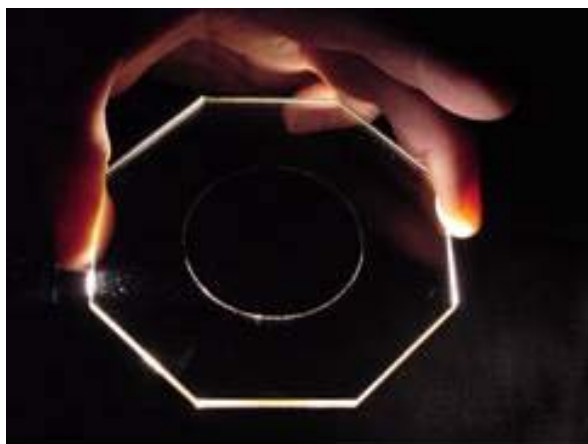
Figure 7: Composite laser disk sliced out of a production billet prior to coating
