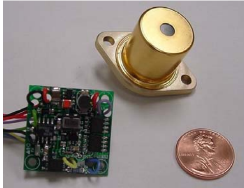
Fig. 1 – Kilowatt class mil-spec high peak power diode pumped Er:Glass laser
